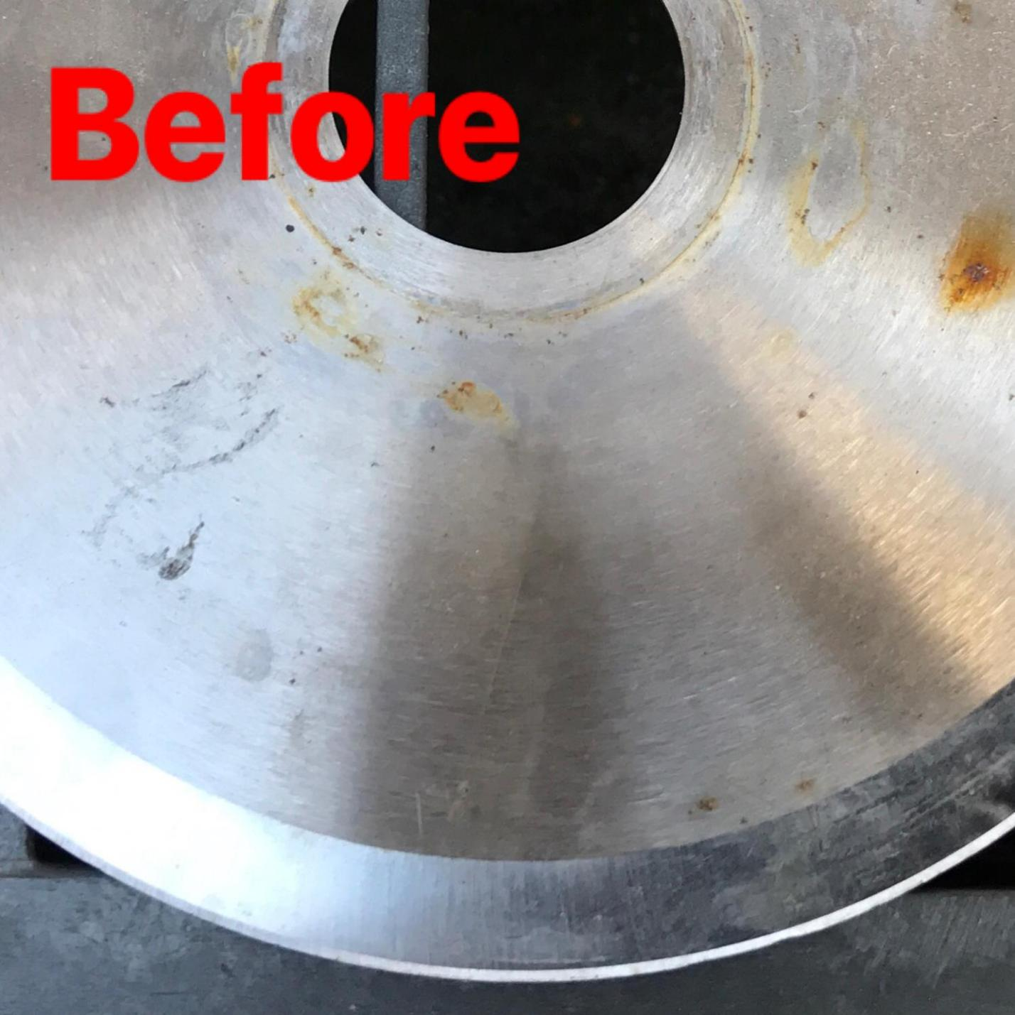
A close-up photograph of a circular metal flange, likely made of aluminum or steel. The surface is heavily worn, showing numerous scratches, scuffs, and several distinct areas of rust, particularly around the central hole and along the outer edge. The lighting is bright, highlighting the texture and damage of the metal.
